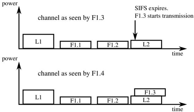
Figure 5: Distributed EDCA bursting problem in case of packet losses.
